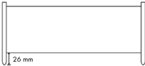
Softline comes with a 25 mm super elliptical shaped edging of solid wood. The distance between the front edge of the end panel and the front edge of the shelf is 26 mm.
