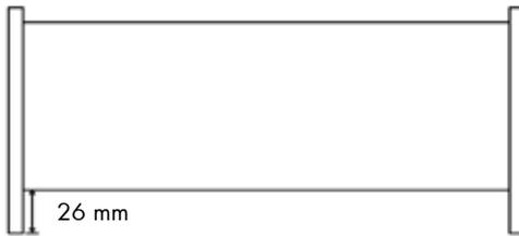
Slimline comes with a 4 mm flat front edge of solid wood. The distance between the front edge of the end panel and the front edge of the shelf is 26 mm.
