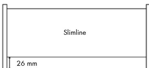
The end panel comes in Softline or Slimline design. The kickplate for height 182 cm is 21 cm and for height 212 cm is 12 cm.
