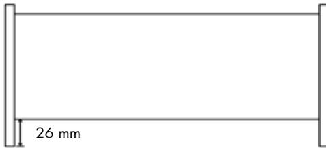
The shelving system has panels with a straight front edge. The wooden shelves are concave on the inside of the circle and convex on the outside of the circle. The inside diameter of full shelving circle is 228.7 cm and the outside diameter of full shelving circle is 357.4 cm.
