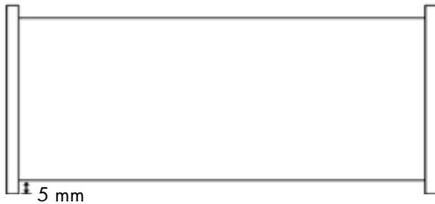
The Frontline end panel has a 4 mm flat front edge of solid wood. The distance between the front edge of the end panel and the front edge of the shelf is 5 mm.
