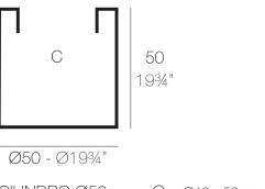
CILINDRO Ø50 CYLINDER Ø1934"  $C = \emptyset 42 \times 50 \text{ cm}$  $C = \emptyset 16\frac{1}{2}" \times 19\frac{3}{4}"$
